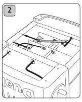
Loosen locking nuts on Unscr retaining plate using a 6.5mm wires. spanner and slide back.
